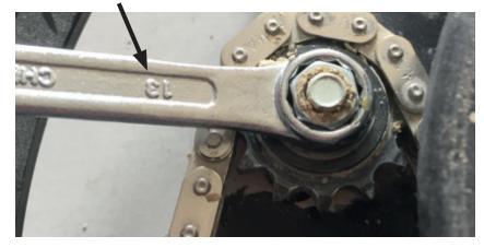
5. Pull the chain tensioning wheel outwards and tighten the nut with the wrench.
