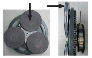
**Clean complete Triple Disc** with compressed air or clean with a damp cloth. (wear safety goggles and wear a dust mask)
